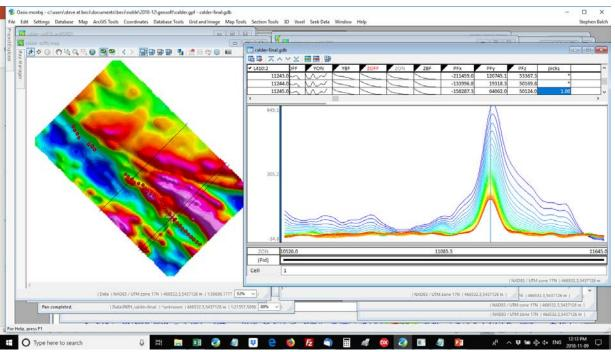
Figure 1: Calder Gold Target - Airborne EM Trend and Profile
