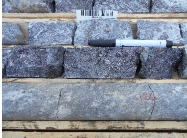
Figure 12b) Low grade graphite in garnet-gneiss (BH16-01)
